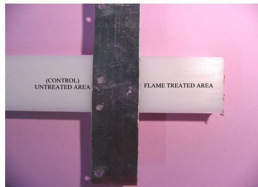
Testing UHMW Plastic for Flame treating efficacy
